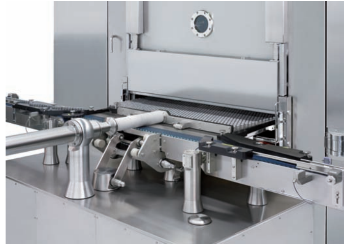
When automatic loading systems are utilized the activity of placing sensors to monitor product temperature becomes extremely difficult.
