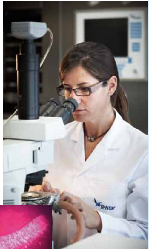
Cryogenic microscope for determination of the collapse temperature.
